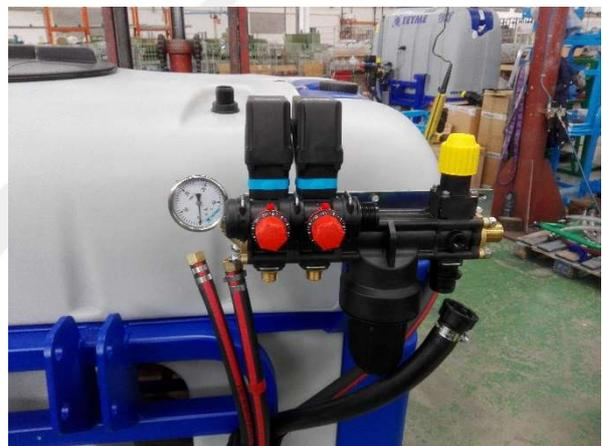
4. Then, remove the stopper of the connection of the tank and connect the transparent hose of the electrical control kit as the picture.
