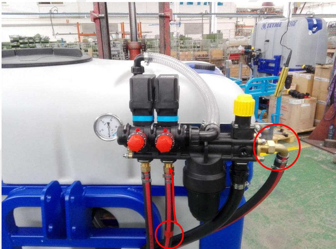
6. To finish, connect the cables of the electric control and test that the controls are opening the correct sides of the spraying.
