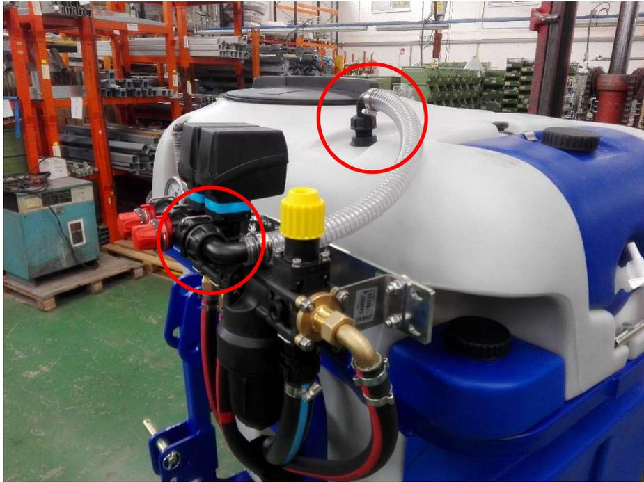
5. Then, connect the two small hoses as the picture. Important! **The hose with the red mark must go to the right way!** The hose with the elbow connection goes as the picture.
